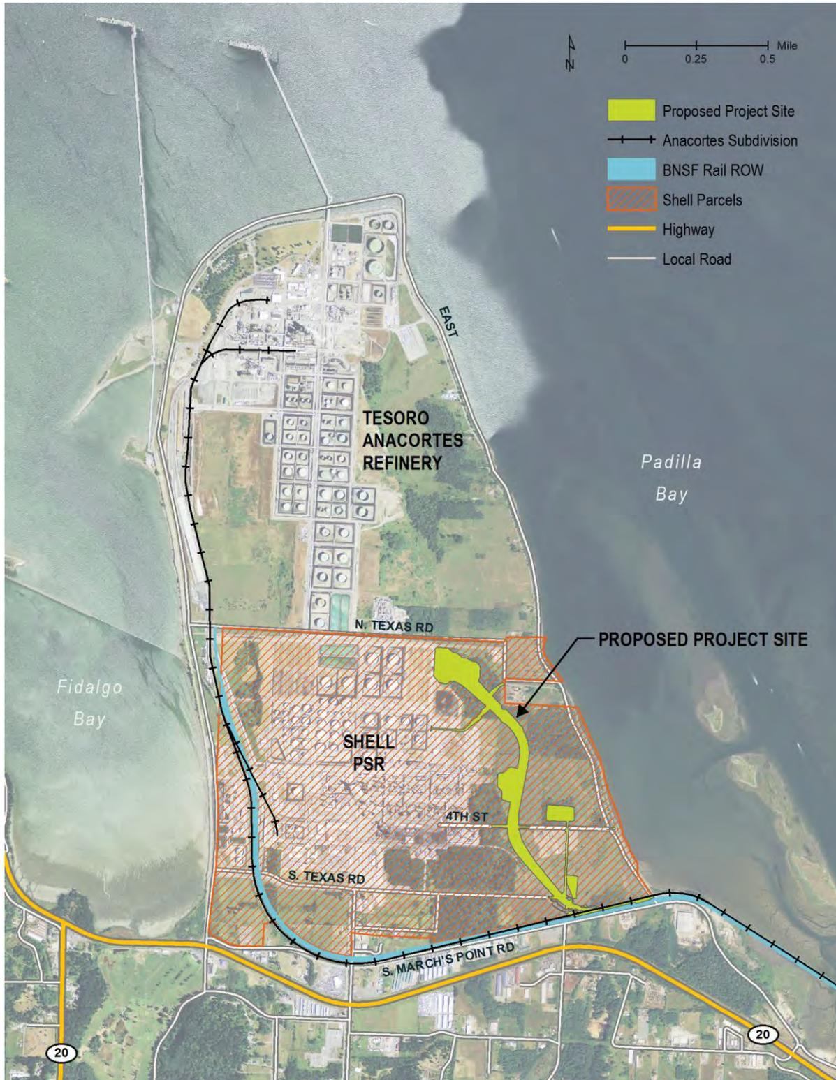
In addition to building the rail spur, the project would include installing equipment and facilities to pump oil from rail cars to existing tanks within the refinery, constructing stormwater detention ponds, and installing safety and spill response measures. Figure ES-3 presents a graphic representation of the key features of the proposed project.
